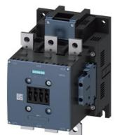
power contactor, AC-3 300 A, 160 kW / 400 V, AC (50-60 Hz) / DC operation 110-127 V AC/DC auxiliary contacts 2 NO + 2 NC 3-pole, frame size S10 busbar connections drive: conventional screw terminal NEMA version
