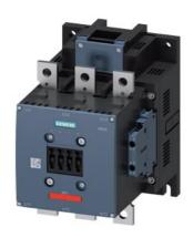
power contactor, AC-3e/AC-3 300 A, 160 kW / 400 V, AC (50-60 Hz) / DC Uc: 23-26 V 3-pole, auxiliary contacts 2 NO + 2 NC permanently mounted drive: conventional main circuit: busbar control and auxiliary circuit: screw terminal
