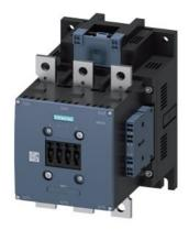
power contactor, AC-3e/AC-3 300 A, 160 kW / 400 V, AC (50-60 Hz) / DC Uc: 200-277 V PLC input 24 V DC 3-pole, auxiliary contacts 2 NO + 2 NC drive: electronic main circuit: busbar control and auxiliary circuit: spring-loaded terminal
