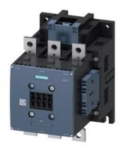
power contactor, AC-3e/AC-3 300 A, 160 kW / 400 V, AC (50-60 Hz) / DC Uc: 96-127 V PLC input 24 V DC 3-pole, auxiliary contacts 2 NO + 2 NC drive: electronic main circuit: busbar control and auxiliary circuit: spring-loaded terminal
