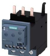
Monitoring relay, can be mounted to Contactor 3RT2, Size S2 basic, analog adjustment Apparent current monitoring 8...80 A, 50...60 Hz, 2-phase Supply 24-240 V AC/DC 1 change-over contact Monitoring for Current overshoot and undershoot Phase failure, Cable break with or without fault buffer ON delay 0-60 s Noise pulse suppression 0-30 s Switching hysteresis 6% Screw connection system
