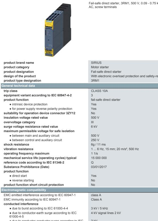
Fail-safe direct starter, 3RM1, 500 V, 0.09 - 0.75 kW, 0.4 - 2 A, 110-230 V
