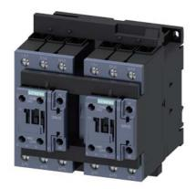
reversing contactor assembly, AC-3e/AC-3, 41 A, 18.5 kW / 400 V, 3-pole, 24 V AC, 50/60 Hz, screw terminal, electrical and mechanical interlock, auxiliary contacts:  $2\times1$  NO
