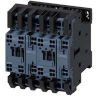
reversing contactor assembly, AC-3e/AC-3, 32 A, 15 kW / 400 V, 3-pole, 110 V AC, 50 Hz / 120 V, 60 Hz, spring-loaded terminal, electrical and mechanical interlock, auxiliary contacts:  $2 \times 1 \text{ NO}$
