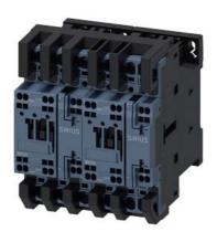
reversing contactor assembly, AC-3e/AC-3, 25 A, 11 kW / 400 V, 3-pole, 24 V AC, 50/60 Hz, spring-loaded terminal, electrical and mechanical interlock, auxiliary contacts: 2 x 1 NO
