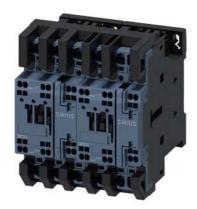
reversing contactor assembly, AC-3e/AC-3, 12 A, 5.5 kW / 400 V, 3-pole, 110 V AC, 50 Hz / 120 V, 60 Hz, spring-loaded terminal, electrical and mechanical interlock, auxiliary contacts: 2 x 1 NO
