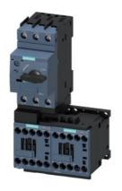
Load feeder fuseless, Reversing duty 400 V AC, Size S00 1.10...1.60 A 24 V DC screw terminal for installation on standard mounting rail (also fulfills type of coordination 1) Type of coordination 2, Iq = 150 kA 1 NC (contactor)
