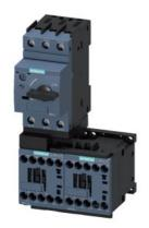
Load feeder fuseless, Reversing duty 400 V AC, Size S00 0.70...1.00 A 24 V DC screw terminal for installation on standard mounting rail (also fulfills type of coordination 1) Type of coordination 2, Iq = 150 kA 1 NC (contactor)
