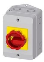
SENTRON, Switch disconnector 3LD, emergency switching-off switch, 3-pole, Iu: 32 A, operating power / at AC-23 A 400 V: 11.5 kW, molded-plastic encapsulation for inch cable gland, rotary operating mechanism, red/yellow
