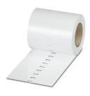
Marker for terminal blocks, Roll, white, unlabeled, can be labeled with: THERMOMARK ROLL 2.0, THERMOMARK ROLL, THERMOMARK ROLL X1, THERMOMARK ROLL MASTER 300/600, THERMOMARK X1.2, THERMOMARK S1.1, perforated, mounting type: snapped, snap into flat marker groove, for terminal block width: 6.2 mm, lettering field size:  $6.35 \times 6.15$  mm, Number of individual labels: 16000
