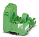
MCR current measuring transducer, for measuring sinusoidal and non-sinusoidal alternating currents, input current 0...400 A, loop-powered output with 4...20 mA
