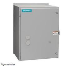
Reversing motor starter, Size 3, Three phase full voltage, Amb. compensate bimetal OLR, Contactor amp rating 90A, 24VAC 50-60Hz coil, Non-combination type, Enclosure type 12, Dust/drip proof for indoors
