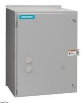
Reversing motor starter, Size 3, Three phase full voltage, Amb. compensate bimetal OLR, Contactor amp rating 90A, Non-combination type, Enclosure type 12, Dust/drip proof for indoors
