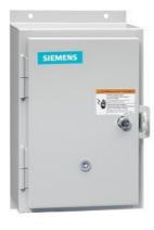
Reversing motor starter, Size 0, Three phase full voltage, Solid-state overload relay, OLR amp range 0.75-3.4A, 110V 50Hz / 120V 60Hz coil, Non-combination type, Enclosure type 12, Dust/drip proof for indoors, Standard width enclosure
