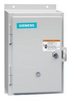
Reversing motor starter, Size 0, Three phase full voltage, Solid-state overload relay, OLR amp range 0.75-3.4A, Non-combination type, Enclosure type 12, Dust/drip proof for indoors, Standard width enclosure
