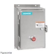
!!! Phased-out product !!! Possible successors include: 22CUC32WG,22CUD32WG,22CUA32WG, 22CUB32WG Reversing motor starter Size 0 Three phase full voltage Amb compensate bimetal OLrelay Contactor amp rating 18Amp Non-combination type Encl NEMA type 4X 304 S-steel Water/dust tight non-corrosive
