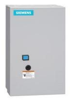
Reversing motor starter, Size 0, Three phase full voltage, Amb. compensate bimetal OLR, Contactor amp rating 18A, 208VAC 60Hz coil, Non-combination type, Enclosure type 1, Indoor general purpose use
