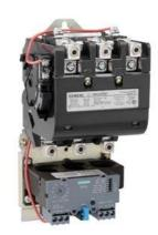
Non-reversing motor starter Size 3 Three phase full voltage Solid-state overload relay OLRelay amp range 25-100A 110-120/220-240VAC 60HZ coil Combination type No enclosure
