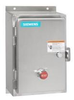
Non-reversing motor starter, Size 3, Three phase full voltage, Amb. compensate bimetal OLR, Contactor amp rating 90A, Non-combination type, Encl. type 4X 304 S. Steel, Water/dust tight noncorrosive
