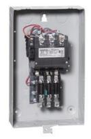
Non-reversing motor starter, Size 2, Three phase full voltage, Amb. compensate bimetal OLR, Contactor amp rating 45A, Non-combination type, Enclosure type 1, Indoor general purpose use
