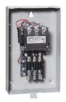
Non-reversing motor starter, Size 2, Three phase full voltage, Amb. compensate bimetal OLR, Contactor amp rating 45A, 110V 50Hz / 120V 60Hz coil, Noncombination type, Enclosure type 1, Indoor general purpose use
