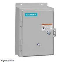
Non-reversing motor starter, Size 2, Three phase full voltage, Amb. compensate bimetal OLR, Contactor amp rating 45A, Non-combination type, Enclosure type 12, Dust/drip proof for indoors
