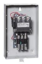
Non-reversing motor starter, Size 2, Single Phase, 2-Pole, Amb. compensate bimetal OLR, Contactor amp rating 45A, 208VAC 60Hz coil, Non-combination type, Enclosure type 1, Indoor general purpose use
